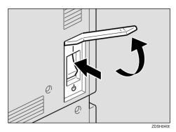
**1** Turn on the operation switch. The On indicator should light.
